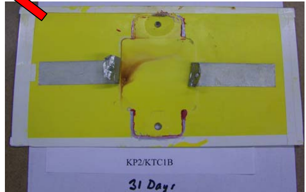
Figure 8. CHM EIS results of two nominally identical panels. One panel (top curve) exhibited a slow decrease in impedance. After 56 days, the panel (upper right) showed no corrosion except at one corner near or under the tape along the panel edge. The other panel (lower curve) exhibited a more rapid decrease in impedance. After 31 days, the panel (right) showed corrosion underneath the mounted CHM.
