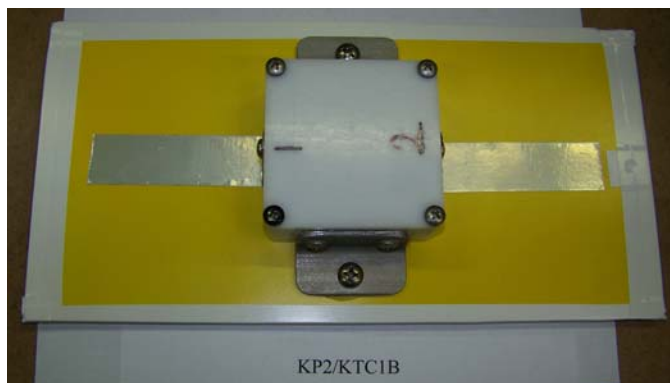
Figure 4. Painted panel with mounted CHM and tape electrodes.
