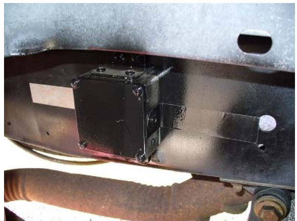
Figure 9. CHM mounted on the frame in a wheel well of a pick-up truck.
